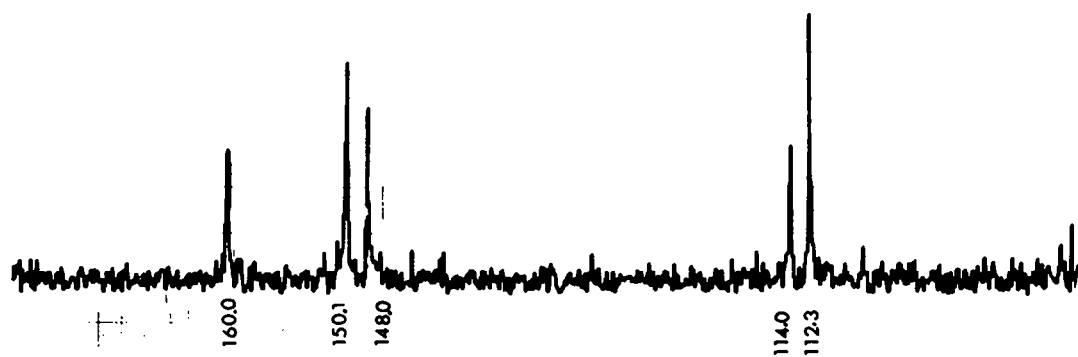
Fig. 3. 22.63 MHz ^1\text{H} -decoupled ^{13}\text{C} spectrum of 3\alpha in \text{DMSO}-d_6 solution; shifts in ppm downfield from TMS.
